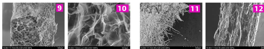
The SEM revealed that paper has fibers randomly oriented in planes parallel to the surface, as seen in the on-edge view (Figure 12). This view also shows the PLA coating on the right, which appears to be around 30µm thick. The first micrograph (Figure 11) hints at some of the paper's mechanical properties, showing the separation and alignment of the fibers around the fracture. The appearance of the ends of the fibers suggests that some broke and some were pulled apart.
